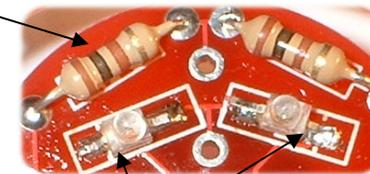
Flatten out the two leads on the LED and solder them to the pad's where the "eyes" on your happy face would go. The Negative side of the LED MUST go on the same side as the white bar on the silkscreen. ( Toward the RIGHT side in this picture. )
