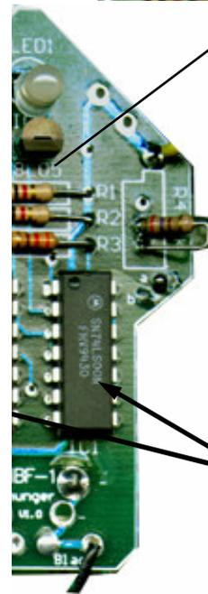
This is the correct way to insert the integrated circuits.
