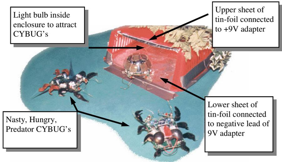
Here's a simple feeding station with a small CYBUG coming out to the waiting claws of two predator CYBUG's ( That's another kit! ) Notice that the feeding station is nothing more than a pair of horizontal sheets of aluminum or tin foil, separated by the height of a small box!
