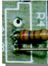
Resistors R4 and R5 must be soldered across the two holes ( pads ) as shown.
